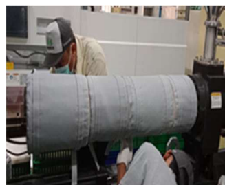
Cylinder with thermal insulation cover
